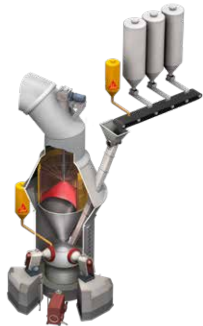
Vertical roller mill
