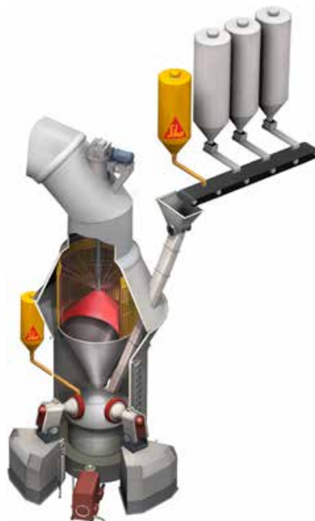
Vertical roller mill.
